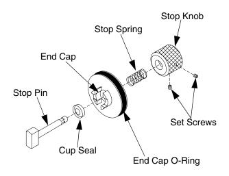
Fig. 14. Safety Stop Assembly
