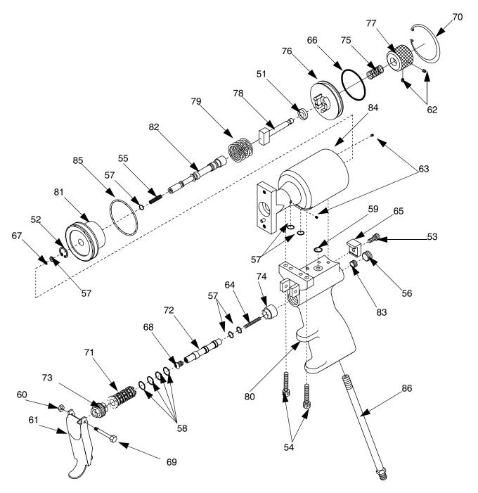
Fig. 19: GAP Pro Handle Assembly
