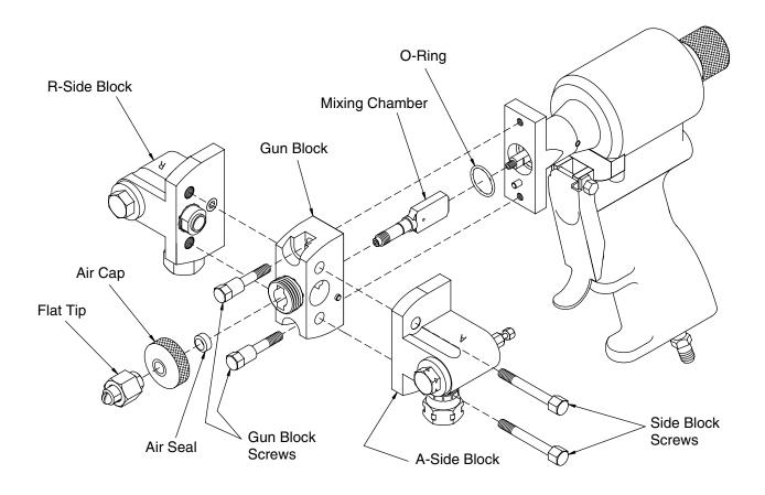
Fig. 10. Mixing Chamber and Gun Block
