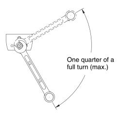
Fig. 8. Tighten Check Valve Retainer
