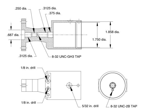
Fig. 16: Air Cylinder Air Passages
