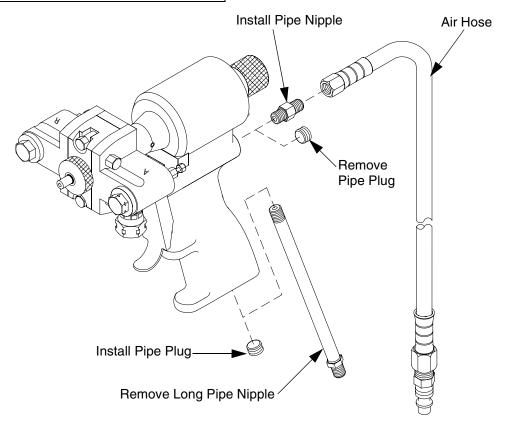
Fig. 6. Air Hose Configuration
