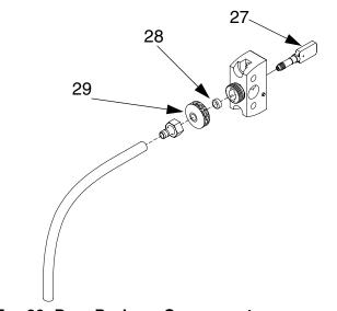
Fig. 20: Pour Package Components
