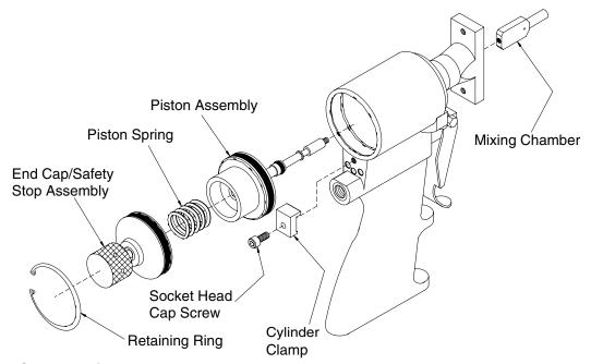
Fig. 11. End Cap and Piston Assembly
