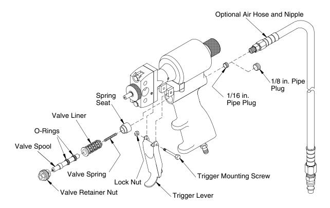
Fig. 15. Trigger/Air Valve Assembly
