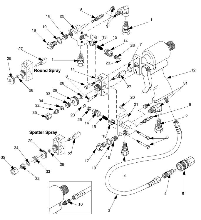
Fig. 18: GAP Pro Final Assembly
