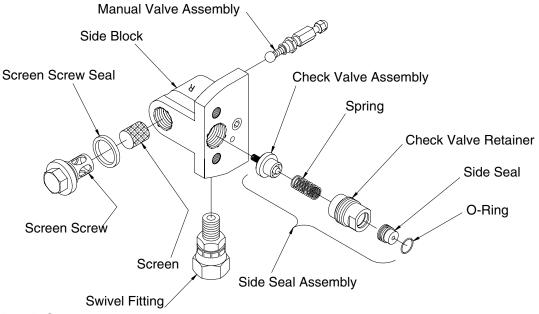
Fig. 7. Side Block Components
